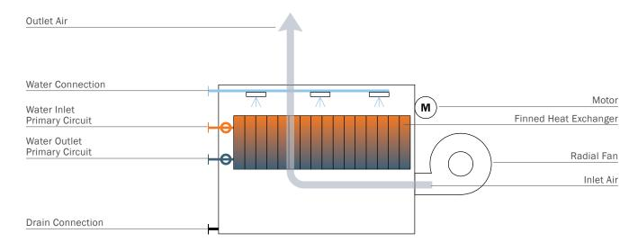
HYBRID EVAPORATIVE COOLER VHK By fitting a fin cooling package to the VK evaporative cooler, a dry cooling element is combined with wet cooling and thus achieves a higher dry cooling performance compared with the classic evaporative cooler. This model of the VK with hybrid design is used when the cooling load is to be discharged air-cooled at cool ambient temperatures without having to forego the low re-cooling temperature at high ambient air temperatures. ◄
